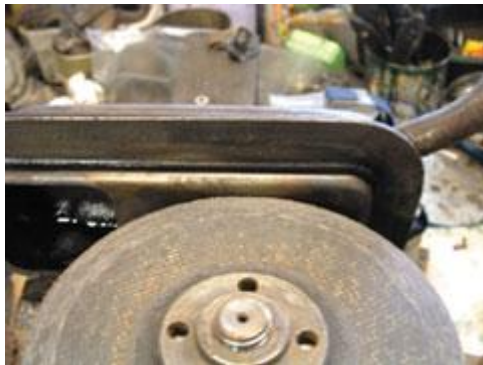
Carefully hold the breather in a vice and use a very thin cutting disc to open it up
