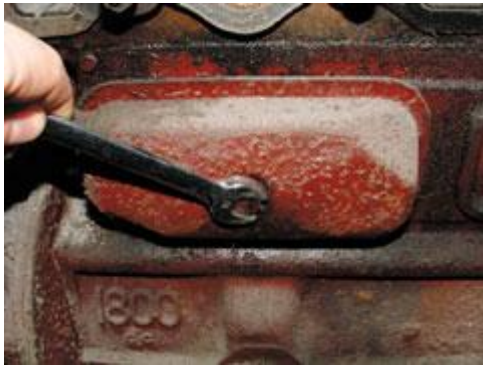
Removing the breather from the side of the engine block
