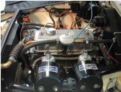
Early engine with 'mushroom' type valve on top of the inlet manifold
