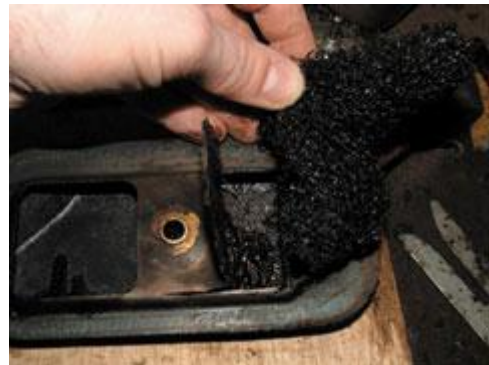
Bend the 'tab' back once cut to reveal the gauze of the breather
