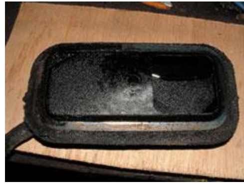
Dirty and partially blocked internal of the crankcase breather
