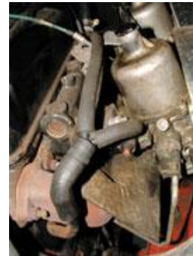
Early engine with 'mushroom' type valve on top of the inlet manifold
