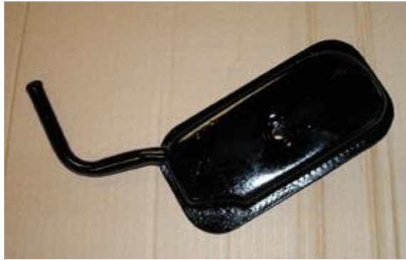
The whole assembly, once painted, can be bolted back on to the block using a new gasket and sealer
