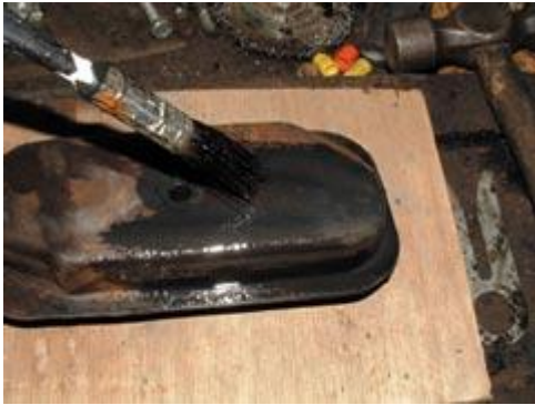
Repainting the breather
