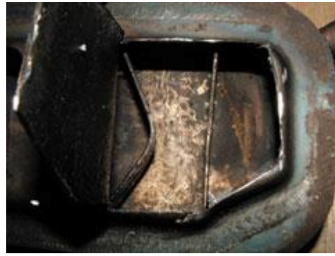
The inside need to be thoroughly cleaned out, including the pipe part. Note the metal strips to help retain the gauze in place
